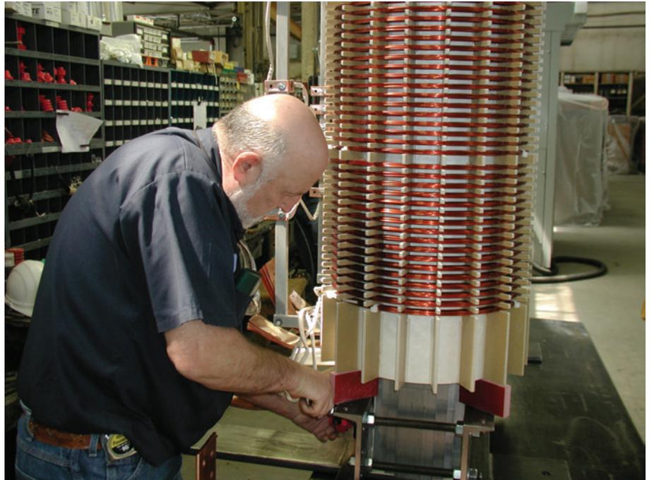
Electric Service Company specializes in emergency replacement. For mission critical applications, transformers can be prepped for shipping within a matter of hours. But to ensure a rapid return to operation, any replacement transformer must duplicate "form, fit and function" as much as possible.
